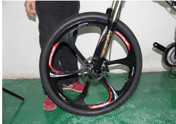
d. Aim the brake disc to the brake device
